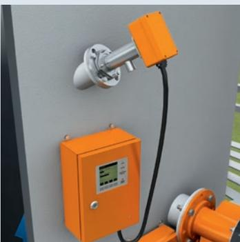
Stack gas flowmeters are often used to determine the mass emissions from combustion sources. The FLOWSIC100 M-AC ultrasonic flow monitor is especially suited for stacks with medium diameter and offers superior accuracy of measurement to meet rigorous environmental standards. It includes internal air cooling of the sensor heads in order to allow the accurate ultrasonic instruments to be used in high temperatures up to +450 °C (+840 °F).
