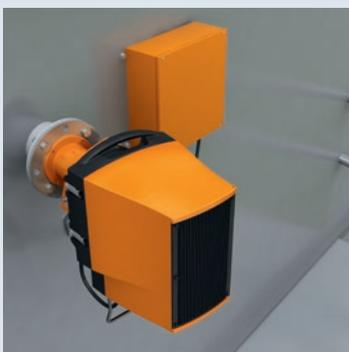
The GM32 in-situ gas analyzer measures continuously low levels of NO<sub>x</sub> directly, fast and without gas sampling and transport. Using the cross duct version, the entire HRSG duct can be used as the active measuring path enabling measurement of very low concentrations of pollutants.
