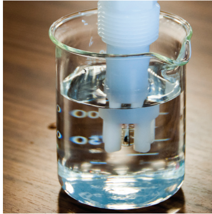
A pH sensor being kept wet in tap water
