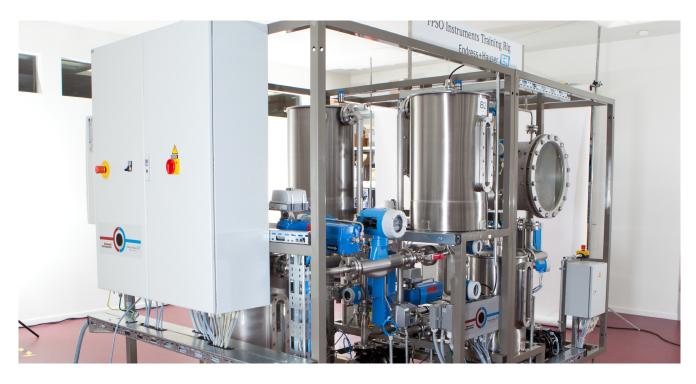
The FPSO training rig simulates the production process on a floating production storage and offloading facility
